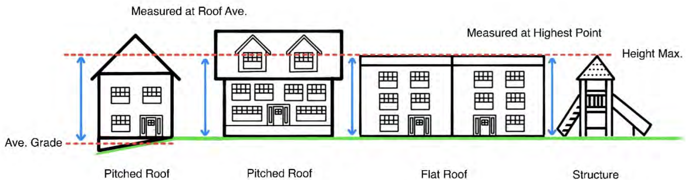
Figure 3-1 Building and Structure Measurements
